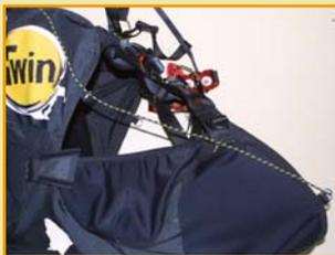
In case you would like to replace the system, check carefully that the strings are linked through all the pulleys of the harness.
