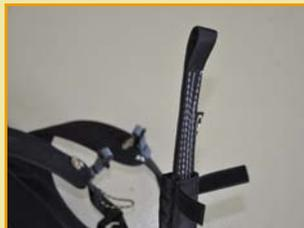
14) Now you can link the riser into the carabiner on the tandem spreader bars.
