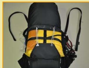
6) Using the strings from the handy kit, start closing the flaps of the container (strings are delivered in the handy kit).
